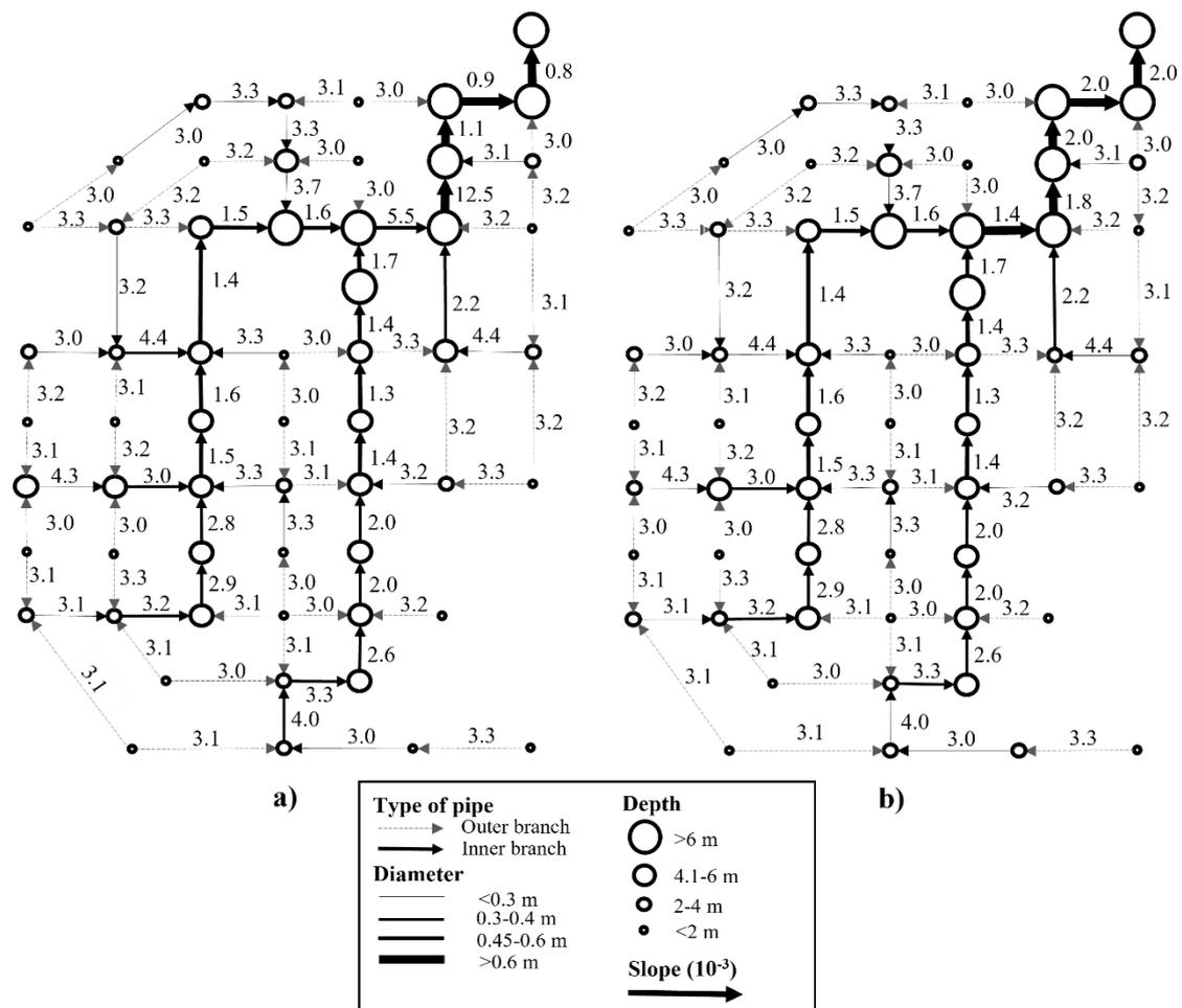
Figure 6. Scheme (not to scale) of the best design of the benchmark network proposed by Li and Matthew [34] with (a) their cost function and (b) the cost function of Maurer et al. [47].
