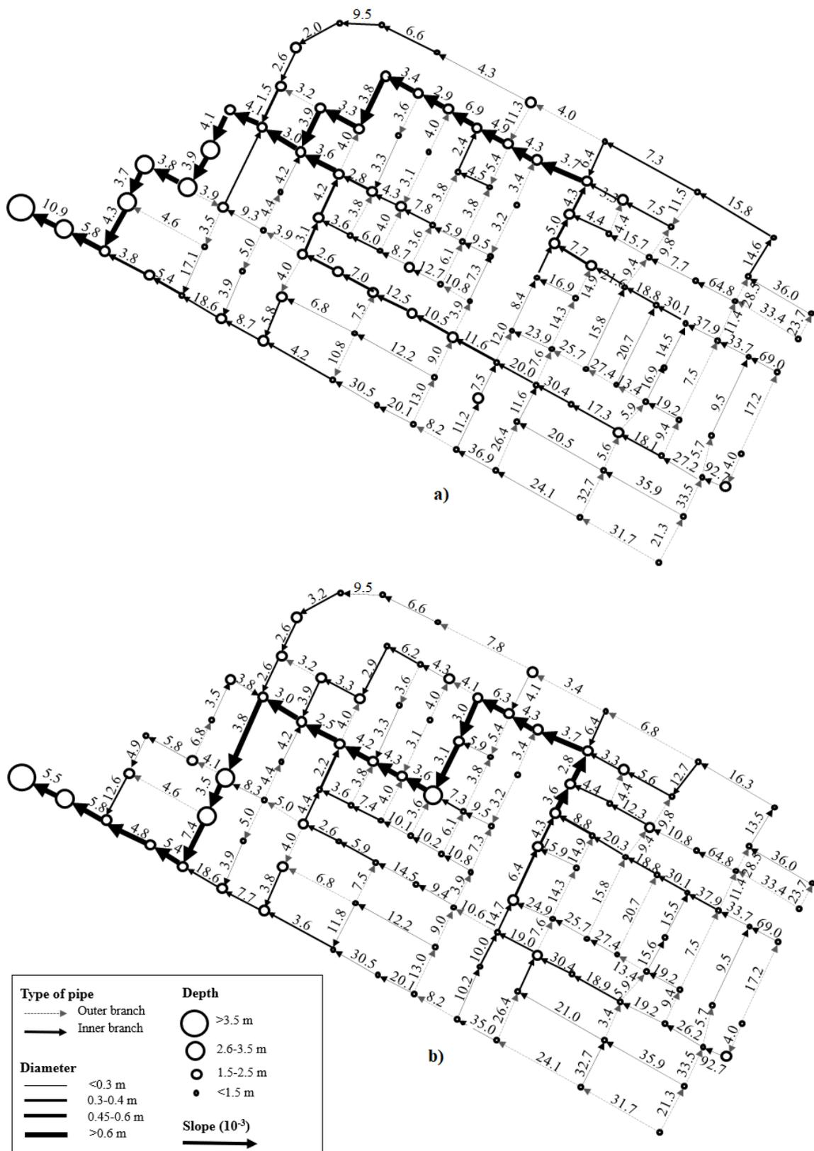
**Figure 8.** Scheme (not to scale) of the best design of the benchmark network proposed by Duque et al. [45] with (a) the cost function of Li and Matthew [34] and (b) the cost function of Maurer et al. [47].
