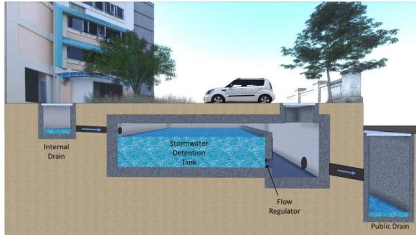
Figure 2.1.1 Schematic diagram of an underground detention tank
