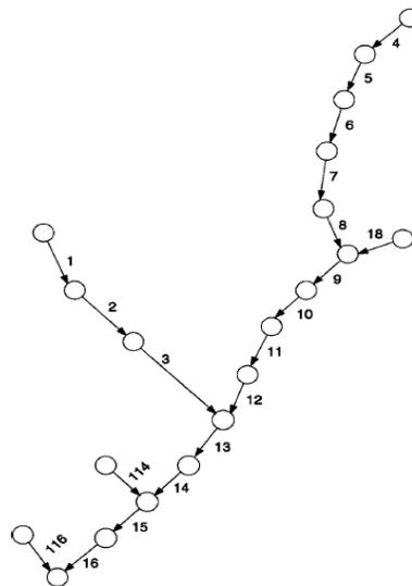
Fig. 3. Storm drainage system diagram
